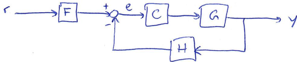
$$\text{error signal: } e = Fr - Hy \quad \left. \begin{array}{l} \\ \end{array} \right\}$$
