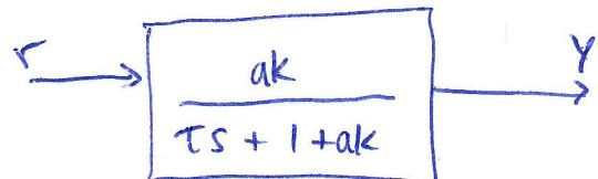
$$\left. \begin{array}{l} \text{New gain: } \frac{ak}{ak + 1} \\ \text{New time constant: } \frac{\tau}{1 + ak} \end{array} \right\}$$
