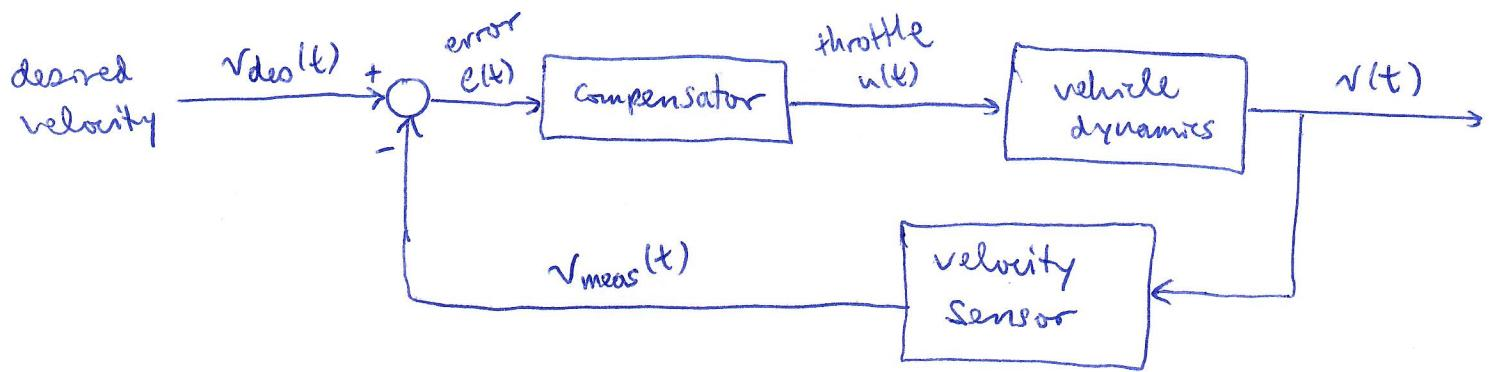
The compensator acts on the error ( $v_{des}(t) - v(t)$ ). In general, the compensator and sensor can have their own dynamics. Here is a general architecture for the tracking problem:
