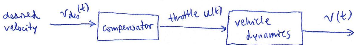
The compensator converts a velocity into a throttle amount (how much the pedal is pressed). What we expect:
